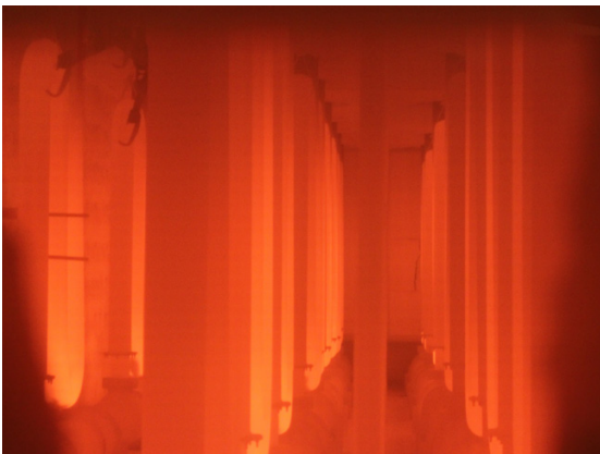
Glass is fused to steel at 1500°F to form a chemical bond.
