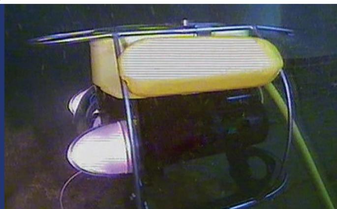
**ROV navigating around the tank**
