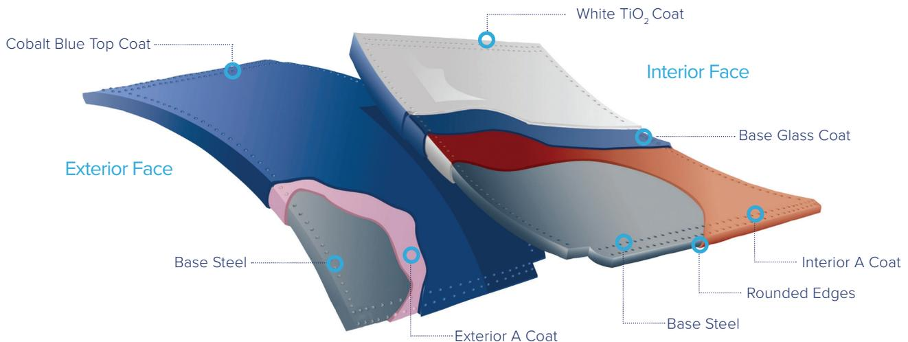
Vitrium™ is the world's leading glass-fused-to-steel coating for bolted storage tanks and has been proven in the field for more than 67 years. CST's Vitrium coating technology enhanced with titanium dioxide (TiO<sub>2</sub>) is applied in a 3-coat, 1-fire (3c1f) process procedure. Vitrium is also produced in a 3-coat, 2-fire (3c2f) process primarily when special colors are requested or thicker layers of glass are required.
