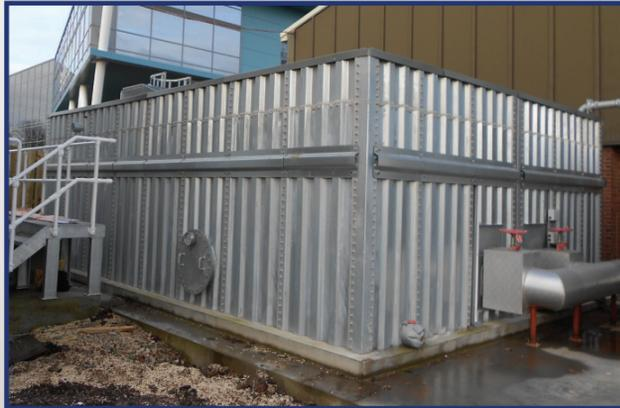
VersaTank is manufactured from corrugated 3mm hot dipped galvanised steel sheets 2.5m high x 1.0m long conforming to BS EN ISO 1461:1999. Heights up to 3.0m are available.
