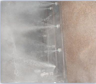
Our proprietary OptiBond Epoxy Coating System provides excellent corrosion resistance and long tank life for the finest epoxy coating available in the liquid tank industry. In the process, parts are degreased and rinsed, hot air dried and pre-heated at an optimum temperature.
