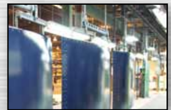
Stage 4: Every glass-fused-to-steel-sheet is high voltage dry tested to be holiday free before shipment and prepared for shipment
