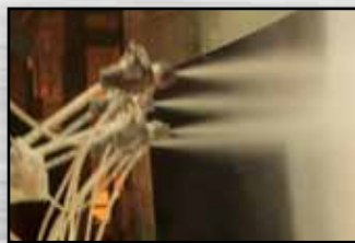
Stage 2: Panels are coated with Vitrium™ glass coating
