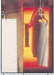
at temperatures of 1500 degrees Fahrenheit to fuse the glass to steel, the physical characteristics and corrosion resistance of Aquastore glass coatings have been thoroughly tested and documented. Our tank systems are ANSI/ NSF Standard 61 certified for potable water contact and conform to AWWA D-103 specifications.
